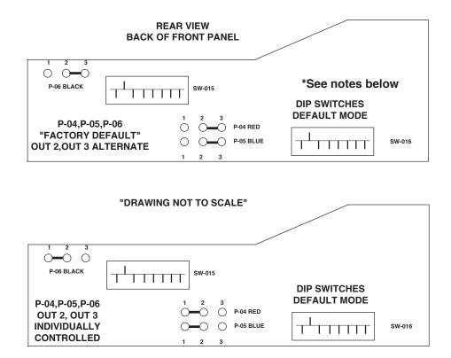
Jumpers marked P-04, P-05, P-06 are used to change from the default mode where OUT 2 and OUT 3 alternate interlocked or are individually (push on, push off) controlled. To set OUT 2 and OUT 3 to individually (push on, push off) mode refer to drawing for jumper configuration.
