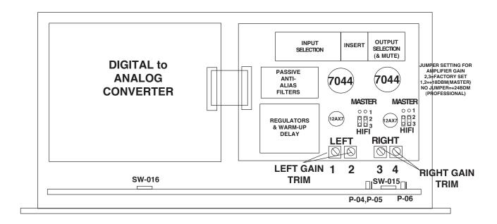
The gain of the Wave's tube stages are set at the factory. There are only 4 trimmers (2 per channel) but because the input to the line amplifier is balanced and it is a minimum feedback design, it requires a trimmer for each phase or leg. So both trimmers affect the gain and the "balance" of the two trimmers affect common mode rejection. Yes, this could have been made more convenient, but it would have compromised some sonic performance.
