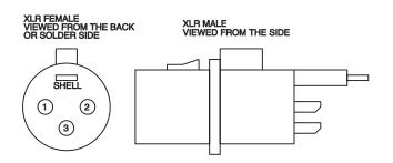
MANLEY GEAR - THIS PAGE CAME WITH GEAR WITH TRUE TRANSFORMER BALANCED XLR INPUTS AND OUTPUTS. ANY 1/4" JACKS ARE UNBALANCED (NO TRANSFORMER). TRANSFORMERS PROVIDE THE MOST "FORGIVING & FLEXIBLE" INTERFACES. OLDER MANLEY GEAR MAY NOT BE BALANCED OR PIN 2 = HOT. CHECK THE ORIGINAL MANUAL.
