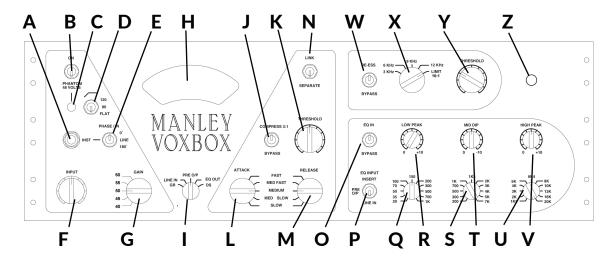
A. INSTRUMENT INPUT: 100 kOhm input impedance. The PHASE switch should be in the middle position to use this input so that the mic input transformer is disconnected. Inserting a phone jack here will interrupt the back panel LINE INPUT. Compression will lower this impedance and can cause some HF loss on guitars but a few dB of compression is OK. Two ways around this are use a preamp or effects pedal between this input and the guitar or use the limiter part of the de-esser.
