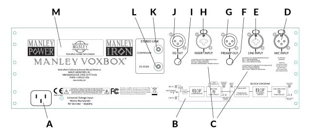
A. IEC POWER CONNECTOR: Use the IEC detachable power cable that was packed with the VOXBOX. The third pin ground is connected to the chassis internally.
