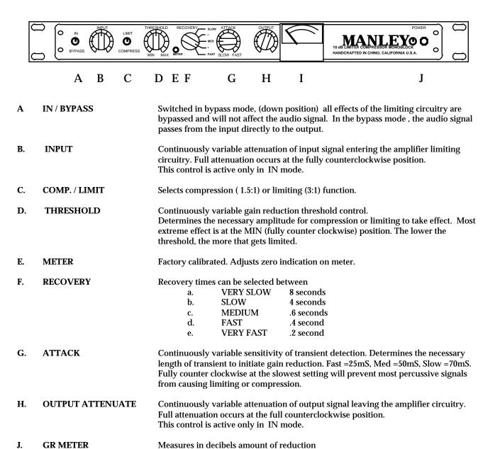
Power is supplied to the unit when switched UP. LED will illuminate
