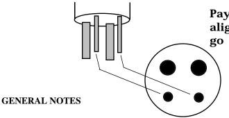
Pay special attention to pin alignment! The 2 small pins must go into the 2 small socket holes.
