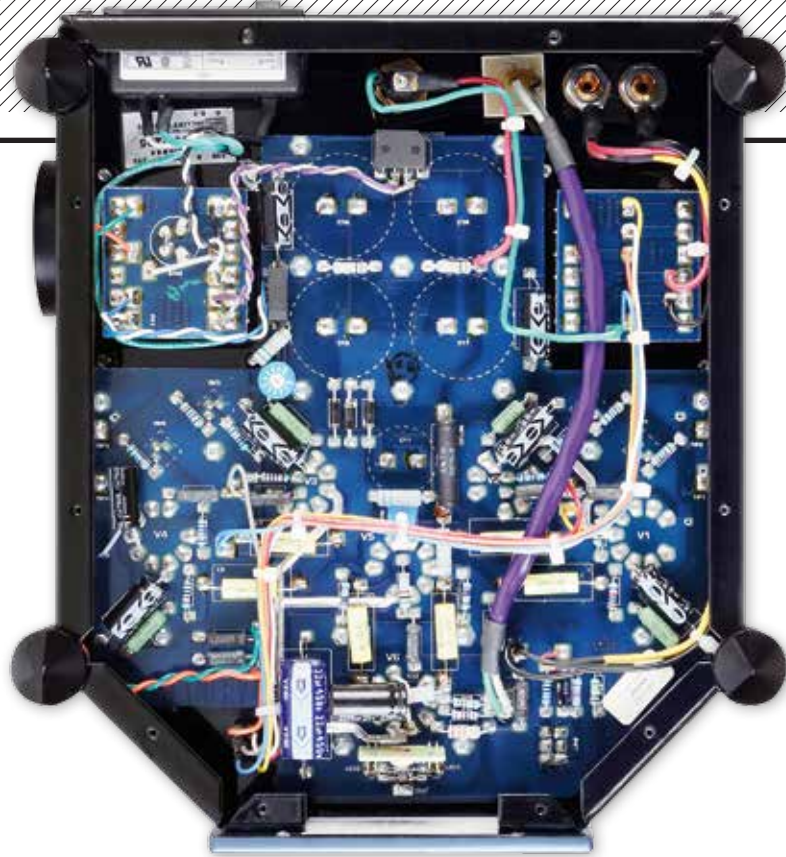
ABOVE: Under the Mahi, revealing a mix of PCB tracks and point-to-point wiring. Two transformers are used, one [top left] for the PSU [top centre] and the other a Manley-custom design optimised for the amplifier's ~50ohm speaker output [top right]
