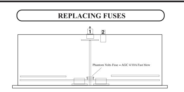
Changing the fuse is easy and can be done without any tools and while the DVC is still in a rack.
