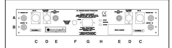
A) PREAMP OUT. This balanced output comes directly from the mike pre and allows you to use the mike pre separate from the limiter. Inserting a TRS plug into this jack breaks the normal signal path between the mike pre output and the limiter input. TIP= +, hot or positive going signal
