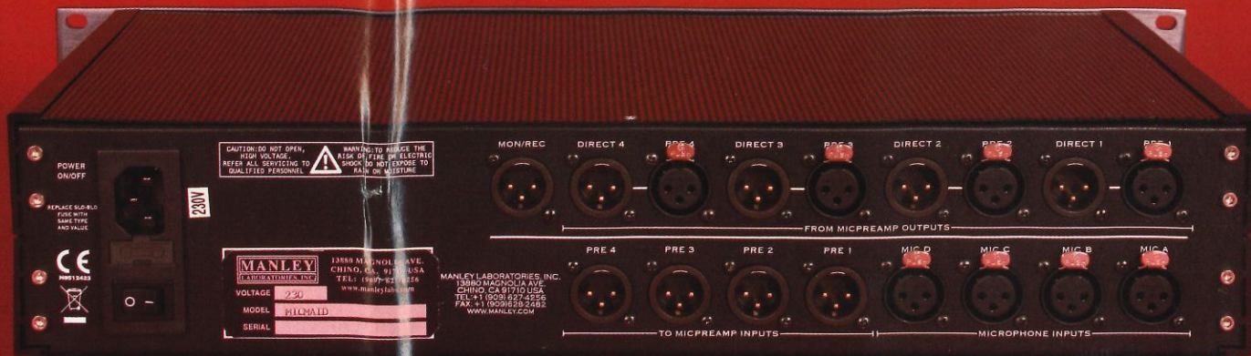
As you'd expect from a device of this type, the rear panel offers quite a set of analogue inputs and outputs, plus a power inlet and on-off switch.
